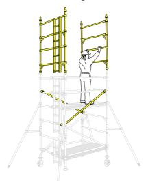
Add two more diagonal braces between the 5th and 7th rungs. If finishing at this height (4.2m platform), reposition the fixed deck to the 8th rung on the tower. Fit a trapdoor deck alongside it, with the hinges towards the outside of the tower, and the trapdoor next to the ladder. Add a single diagonal between the 7th and 9th rungs as shown. Climb up the ladder, and from the protected trapdoor position, fit the guardrails on the 9th and 10th rungs, in that order, on both sides of the tower.
