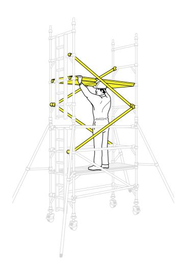
Climb up the inside of the tower and from the protected position of the trapdoor, fit guardrails to the 7th and 8th rungs, (in that order), on both sides of the tower.
