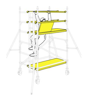
6 Fit the next pair of diagonal braces in opposing directions between the 3rd and 5th rungs add 2 additional end frames.
