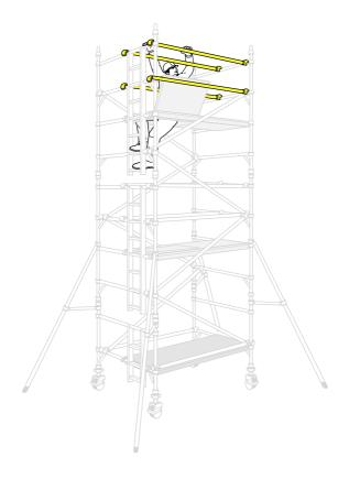
Continue until the required height is reached. Re-position the fixed deck to the required platform height and fit a trapdoor deck alongside it as shown in **stage 7**. Fit a single diagonal at the top of the tower as shown in **stage 7**. Fit the final guardrails as shown in **stage 7**.
