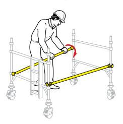
Fit 2 additional end frames ensuring the frame interlock clips are engaged. Fit 2 diagonal braces (blue) in opposing directions, between the 1st and the 3rd rungs. Ensure the frames are vertical and level by checking with a spirit level and setting the adjustable legs as required. Fit stabilisers (see noteson page 30).
