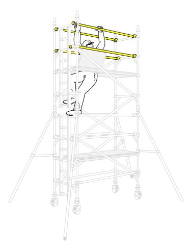
Continue the procedure until the required working height is reached, adding additional pairs of end frames, diagonal braces and fitting trapdoor platforms, as shown on previous steps. At every platform level, add horizontal braces as guardrails from the protected position within the trapdoor, (as shown in **step 5**).
