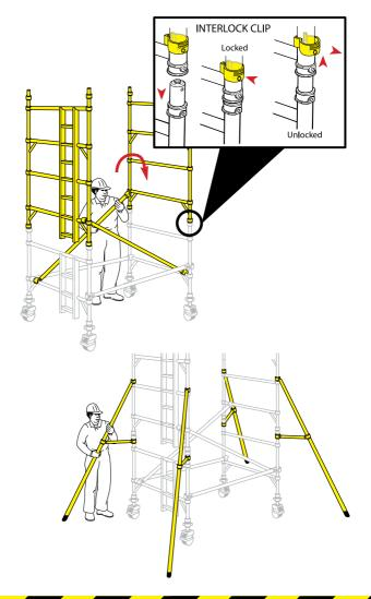
Fit a temporary deck on the lowest rungs. Fit a trapdoor deck on the 4th rung (2.0m) with the trapdoor next to the ladder. Ensure the trapdoor is positioned with the hinges towards the outside of the tower as shown. Climb the ladder and, from the protected trapdoor position, fit guardrails on the 5th and 6th rungs (in that order) on both sides of the platform.
