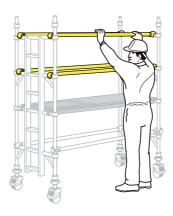
Fit 2 diagonal braces in opposing directions between the 1st and 3rd rungs. Ensure the frames are vertical and level by checking with a spirit level and setting the adjustable legs as necessary. Fit stabilisers (see notes on **page 30**). Fit the next pair of end frames and check the frame interlock clips are engaged.
