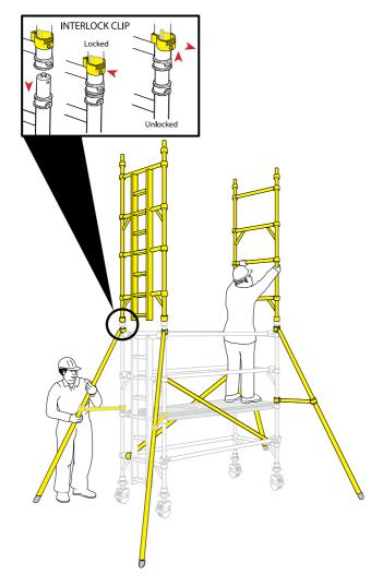
Fit 2 pairs of diagonal braces in opposing directions between the 3rd and 5th rungs and the 5th and7th rungs. Locate a trapdoor deck on the 6th rung, with the trapdoor next to the ladder.
